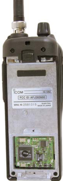
Figure 8—UT-118 digital encoding unit installed in an IC-V82.
