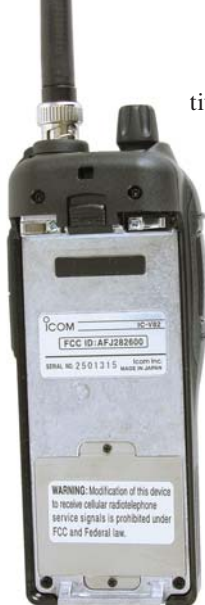
Figure 7—Access door for the UT-118 in the IC-V82 battery compartment.
